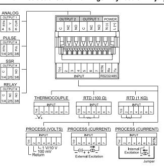
Connect the main power connections as shown in the figure below.
