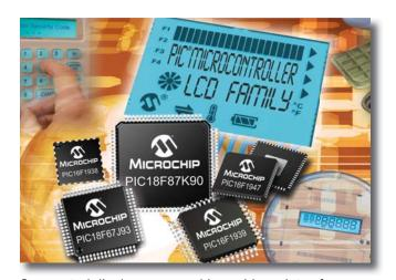
Segmented displays are used in a wide variety of applications, ranging from meters to portable medical devices to thermostats to exercise equipment. PIC microcontrollers with integrated LCD drivers can directly drive segmented displays with letters, numbers, characters
