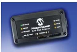
The CAN analyzer development system enables a personal computer (PC) to communicate with the CAN bus. The PC program uses a graphical user interface to enter and display message frames occurring on the target bus.
