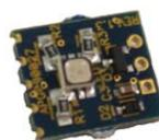
The Automotive Ambient Interior Lighting Module Reference Design demonstrates microcontroller-based control of RGB LED devices. This module can be controlled remotely
