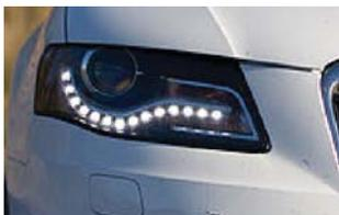
With the advances in technology, LED lighting is being used in both interior and exterior applications within the vehicle. LEDs deliver long life, durability and efficiency. For example
