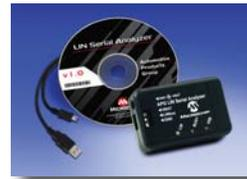
The LIN analyzer development system enables a personal computer (PC) to communicate with the LIN bus. The PC program uses a graphical user interface to enter and display message frames occurring on the target bus.
