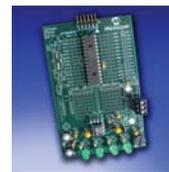
The PICKIT 28-pin LIN demo board enables a quick start in developing and debugging applications with the LIN drivers. The kit includes a 28-pin socket which supports various PIC16F devices, includes a LIN transceiver, plus a generous prototype area with various indicator LEDs and buttons to support the test and debug of the application.
