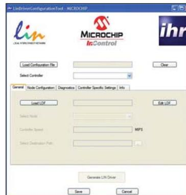
To support the automotive system designers, one of Microchip's design partners, ihr GmbH, has developed LIN Compliant drivers for the PIC16F, PIC18F and PIC24F Family of microcontrollers. The LIN Driver and Configuration tool (LDC) was developed
