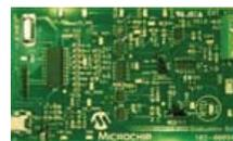
The PT100 RTD Evaluation Board demonstrates how to bias a Resistive Temperature Detector (RTD) and accurately measure temperature. Up to two RTDs can be connected. The
