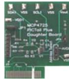
This daughter board demonstrates the MCP4725 (12 bit DAC with non-volatile memory) features using the Explorer 16 Development Board and the PICkit Serial Analyzer.
