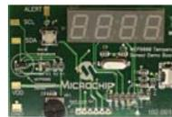
The MCP9800 Temperature Sensor Demo Board demonstrates the sensor's features. Users can connect the demo board to a PC with USB interface and evaluate the sensor performance. The
