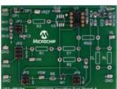
The MCP6XXX Amplifier Evaluation Board 4 is designed to support the inverting integrator circuit.
