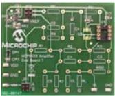
The MCP6XXX Amplifier Evaluation Board 1 is designed to support inverting/non-inverting amplifiers, voltage followers, inverting/non-inverting comparators, inverting/non-inverting differentiators.
