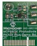
The MCP6031 Photodiode PICtail Plus Demo Board demonstrates how to use a transimpedance amplifier, which consists of MCP6031 high precision op amp and external resistors, to convert photo-current to voltage.
