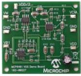
The MCP6V01 Input Offset Demo Board is intended to provide a simple means to measure the MCP6V01/2/3 op amps input offset voltage ( $V_{os}$ ) under a variety of bias conditions. This  $V_{os}$  includes the specified input offset voltage value found in the data
