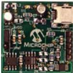
This 1" x 1" board is designed to demonstrate the performance of the MCP3550/1/3 devices in a simple low-cost application. The circuit uses a ratiometric sensor configuration and uses the system power supply as the voltage reference. The
