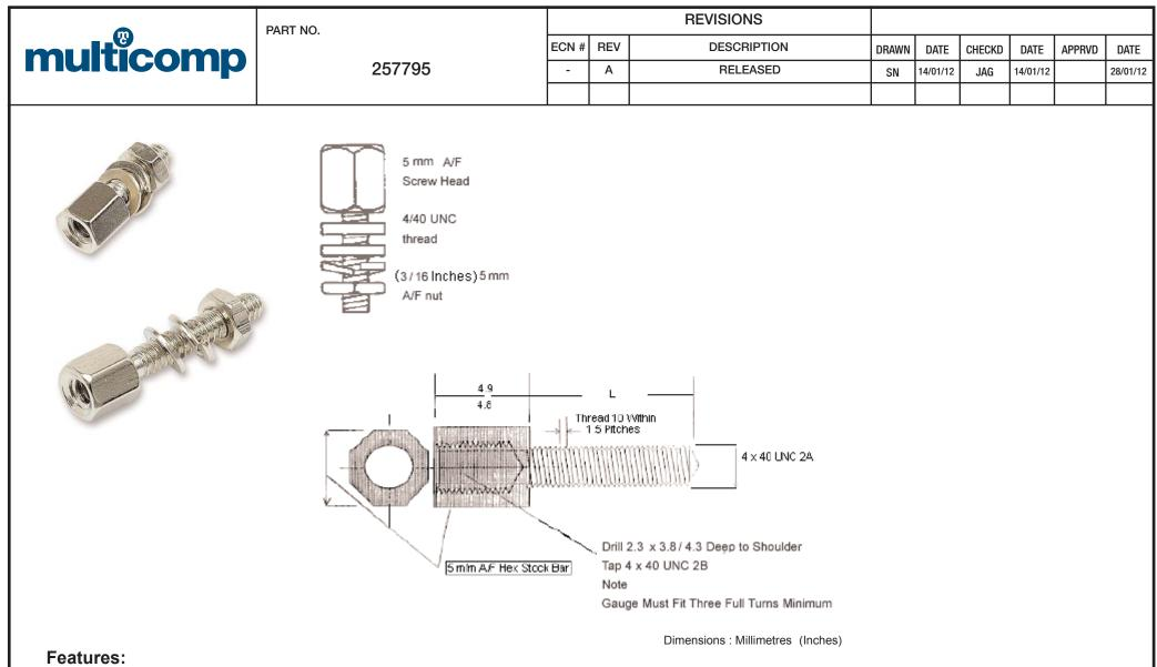
• Bright tin or nickel plating suitable for EMI/RFI shielded 'D' connectors The base of the female screwlocks have chamfered corners to prevent scratching of surface during assembly.
