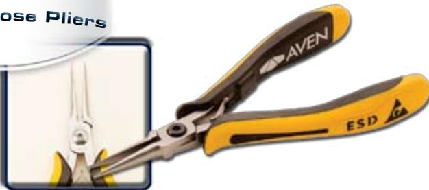
These Pliers have exceptionally fine tips. The outer surface of the jaw is rounded to the shape of smooth half cones. This design increases tool access and allows forming of round loops. All edges of the inner jaws are eased. Tip Dimensions: 1.0mm W x 1.2mm H (.040" x .050")
