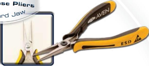
Features very fine tips, "eased" edges of the inner jaw to reduce the risk of damage to the workpiece during forming, and a long jaw for extended gripping power. Available with smooth or serrated jaws. Tip Dimensions: 1.2mm W x 1.4mm H (.050" x .060")
