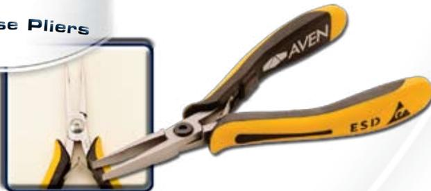
These flat nose pliers have a long jaw and very thin tips. The tip gripping area has a smooth finish. All inner edges are "eased" to reduce the risk of workpiece damage. Flat nose pliers have tips that are 3.5mm (.140") wide.
