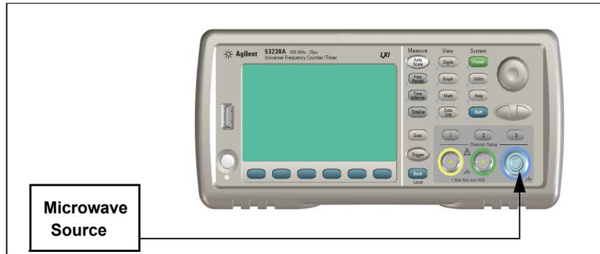
Figure 2-7. Microwave Source Connection to Channel 3
