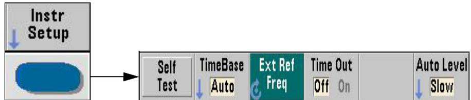
3 Press the Self Test softkey. The display shows:
