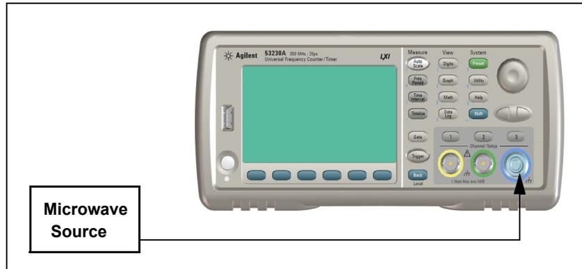
Figure 2-8. Microwave Source Connection to Channel 3
