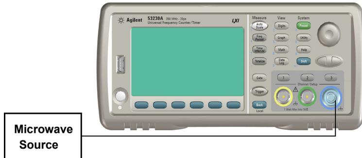
Figure 6-2. Microwave Source Connection to Channel 3
