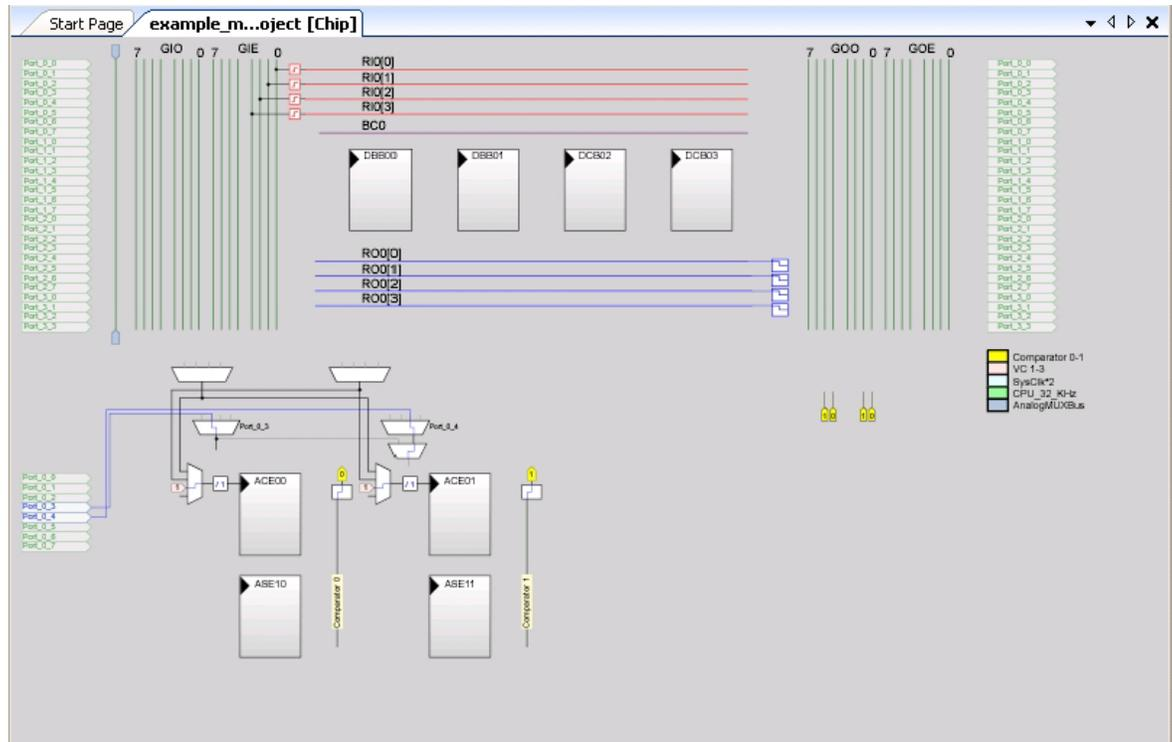
11. Now place and configure the modules required for this design. Connect the modules together and to the pins of the PSoC. In the **User Modules** window, select the **Cap Sensors** folder.
