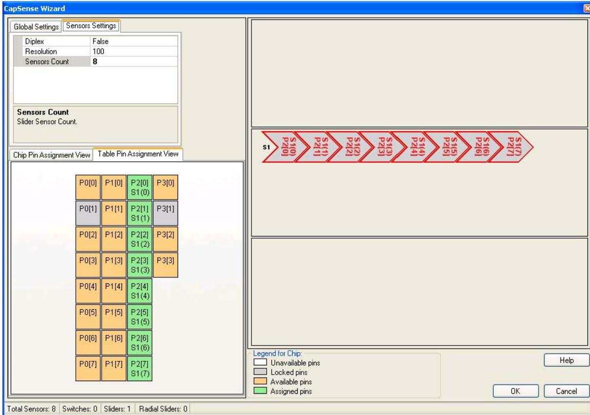
24. All the assigned sensors can be seen in **Chip Pin Assignment View**.
