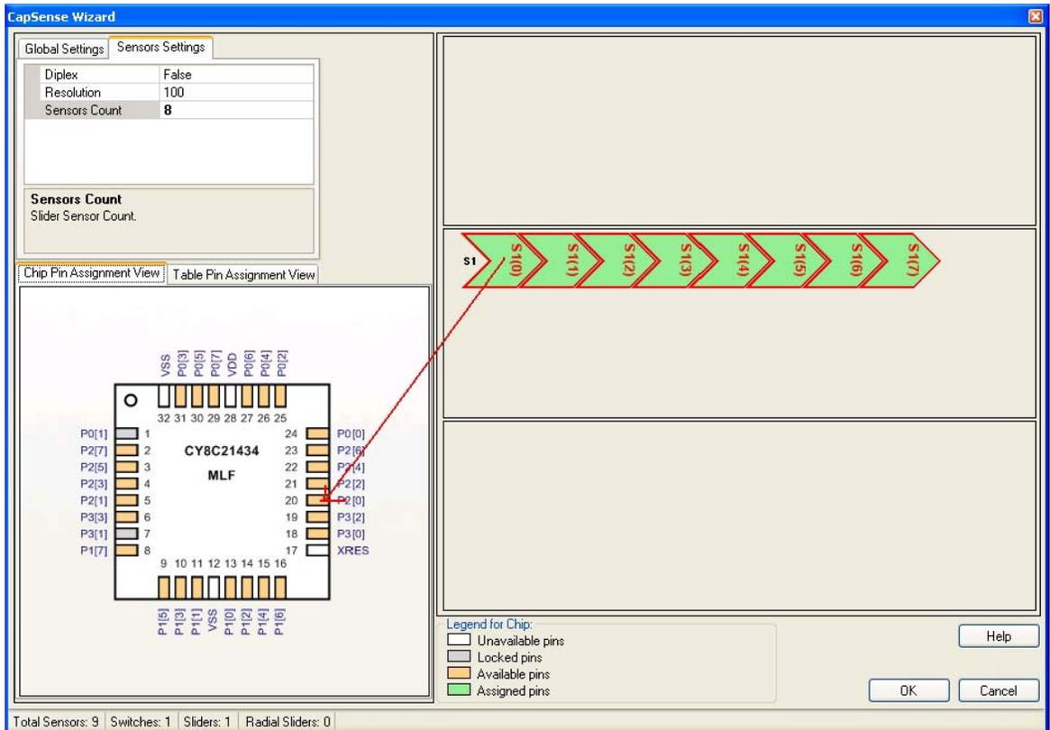
23. Similarly, assign all the sensors from S1(1) through S1(7) to pins P2[1] through P2[7] and click **OK**.
