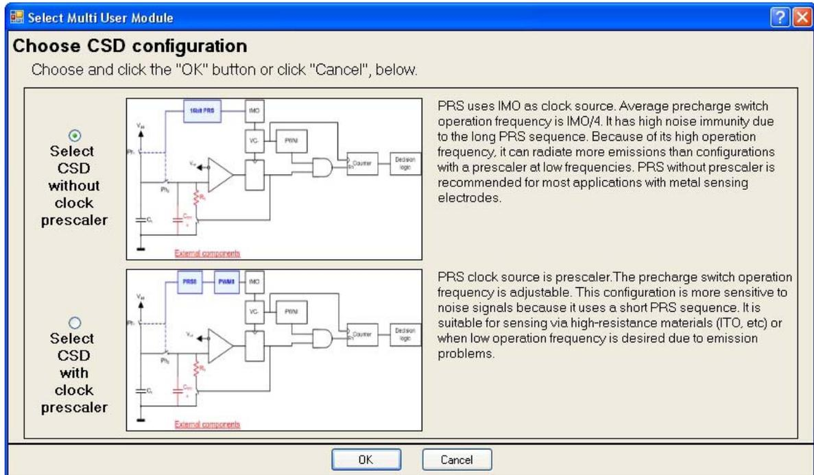
14. The User Module (UM) CSD is placed in the analog and digital blocks respectively.
