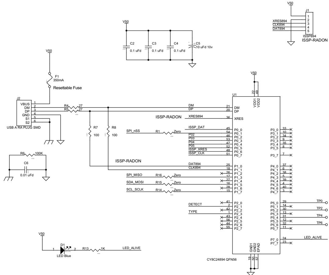
Note that the CY8C24894 PSoC device is the only active component in the entire circuit. This single PSoC handles all communications between the applications, USB, and expansion card interfaces.
