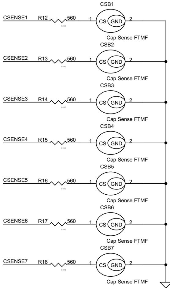
The CY8C21434 PSoC that resides on the FTMF expansion card detects your finger's position on the CapSense touch sensing slider and controls the LEDs output. Adopting capacitive sensing as an interface technology in high-volume, high-visibility applications such as portable media players and mobile handsets has created demand for the same technology in more conventional consumer electronics. Its hardware details are shown in the [Figure 4-7](#).
