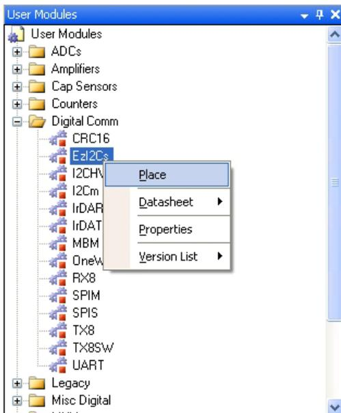
27. The EzI2Cs module does not require any digital or analog blocks for placement. It requires either (configurable) P1[0] and P1[1] or P1[5] and P1[7] port pins to operate as SCL and SDA.
