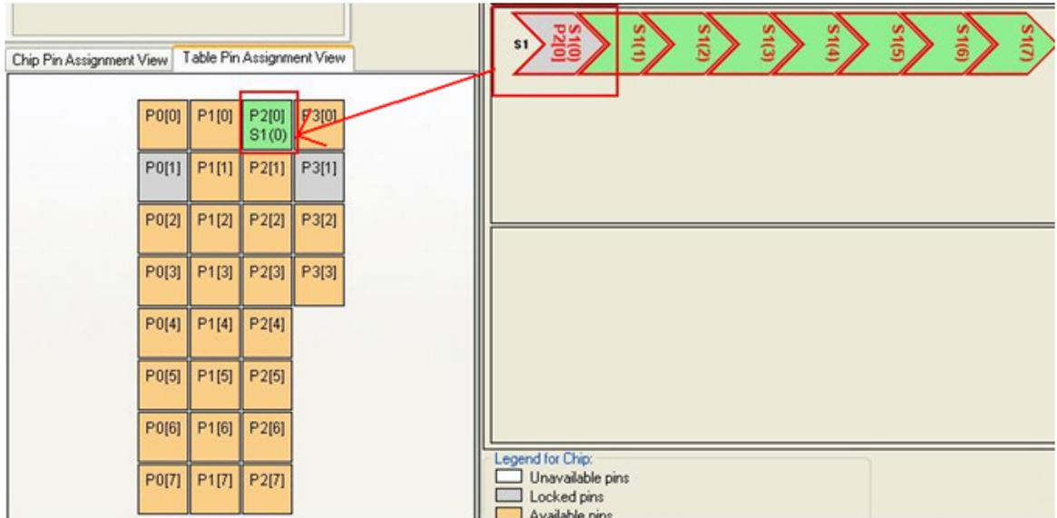
Figure 5-17. S1 (0) Assigned to Pin P2 [0]
