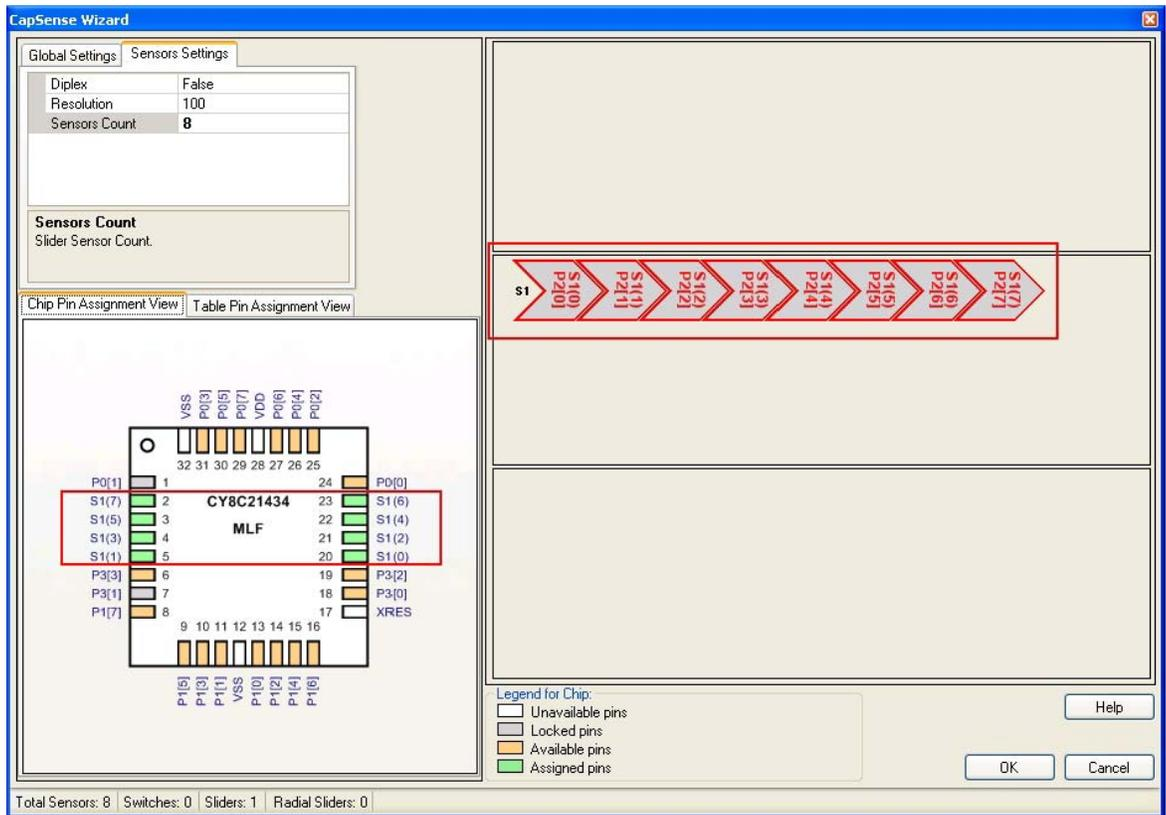
25. After configuration in the **CSD Wizard** window, the pins to which sensors are assigned can be seen in the **Chip Level** diagram.
