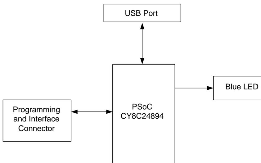
Figure 4-2. System Block Diagram for First Touch Multifunction Card
