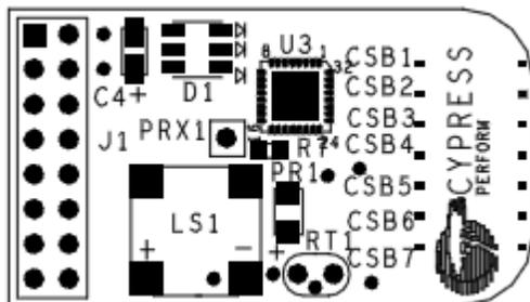
A.2.4 Assembly Drawing of First touch Multifunction Card (Secondary Side)
