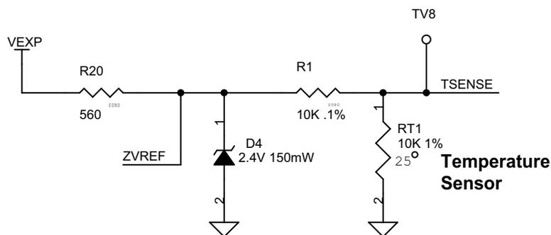
The thermistor is used to measure the temperature and will be given as the input to PSoC. The LEDs are used to represent the different values received from the device. A buzzer can be used as a sound alert when the data goes above or below a certain level.
