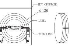
UTP CAT. 5E Cable, Contact Gold Plated (3u), Line Colour Grey; Jacket: LSOH Wiring: 24AWG (7/0.18mm Cu) × 4P; OD: 5.0mm ± 0.15mm; Length: 10.0m Printing: System Cable UTP Cat 5E 4 Pairs 24AWG; Stranded ISO 11801 100MHz (Font: Arial 12, 1 Group / 1M) / LSOH 100% Open, Short & Miswire Test Packing: 1 Pcs / Polybag with Label;
