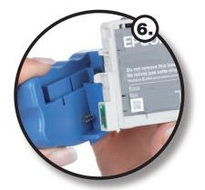
Finally, the ink cartridge chip ink fluid level reading needs to be reset. In order to do this, press the reset device (not included with the refill kit set) pins against the ink cartridge chip contact. After removing the adhesive tape from the ink outlet area, the refilled ink cartridge can then be inserted into the printer. Please be aware of the possibility of ink leakage.
