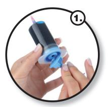
In order to refill an ink cartridge, a syringe filled with ink is required. Open the cap of one of the enclosed ink holders, which also acts as a syringe. Now insert the enclosed blunt needle using a twisting motion into the opening. Hold the lower part of the ink holder with your thumb and forefinger and twist it counter clockwise into the appliance.
