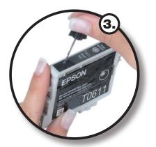
Next, using the tool provided, drill a hole approximately 7 mm deep through the designated opening. Drill carefully, as there are 2 inner walls to drill through.
