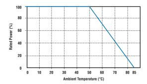
When the ambient temperature exceeds  $50^{\circ}$ C, reduce the rated power and current in accordance with the derating curve shown
