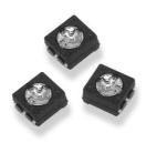
The latest miniaturised sealed trimmer from Citec is the smallest, lightest sealed potentiometer available and the most cost effective. Consuming just 10.5mm² of board real estate, it has been developed specifically for new generation hand held equipment, where double sided component placement is often unavoidable. These 3mm devices are only 1.8mm high. Due to the innovative carbon on polymer technology, the device sets new standards in low cost high reliability electro mechanical components.
