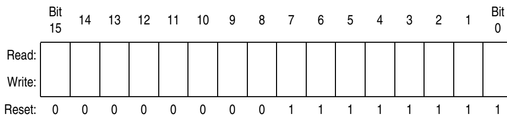
Figure 6-4. Stack Pointer (SP)
