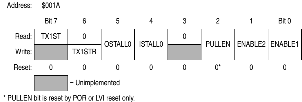
Figure 9-22. USB Control Register 3 (UCR3)
