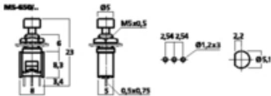
**Momentary mini push-buttons**, 1 x ON/ON, hermetically sealed, print connections. Red (RT) and black (SW). For safety extra-low voltage or signal voltage. Current rating: 0.4A.
