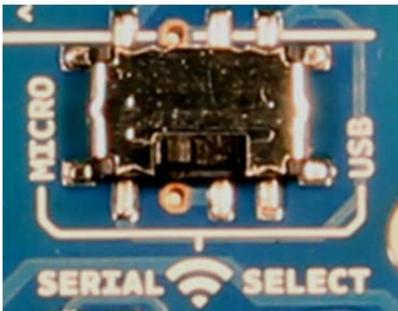
With the switch in the **USB** position, the DOUT pin the wireless module is connected to the RX pin of the USB-to-serial converter, and DIN on the wireless module is connected to the TX pin of the USB-to-serial converter. This means that the module can communicate directly with the computer. The microcontroller on the board will be bypassed. **To use the shield in this mode, you must program the microcontroller with an empty sketch (shown below), or remove it from the board.**
