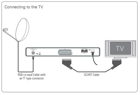
Connect a RG6 co-axial cable fitted with an 'F' type connector from your satellite dish to the 'LNB IN' socket on the back panel of your digital box.
