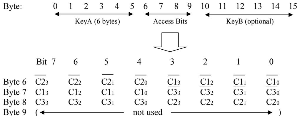
$\overline{C_{xy}}$  = Inverted bit
