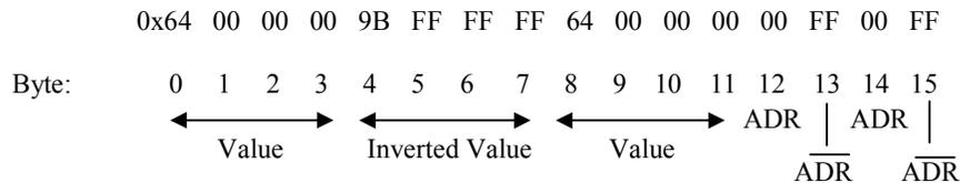
Note that the ADR and inverted ADR block address is part of the required format for the Value Data Structure BUT it is not changed by the Inc, Dec or Transfer commands and exists to allow optional storage of block numbers. For general use, the 0x00 address and 0xFF inverted address can be used to satisfy the structure format. The Inc, Dec and Transfer commands first check the structure format before beginning the operations and the commands fail if the format is not correct.
