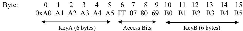
The default access bits (0xFF 07 80 69) define that KeyA must used for all operations and KeyA can never be read, so in the previous example bytes 0 – 5 (keyA) would always read as zeros.
