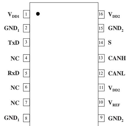
\*NOTE: Pin 11 is not internally connected to pin 16; both should be connected to the V<sub>DD2</sub> power supply for normal operation.
