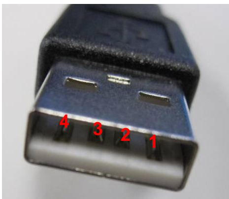
Figure 14. USB Connector on Micro-fit ® USB Cable
