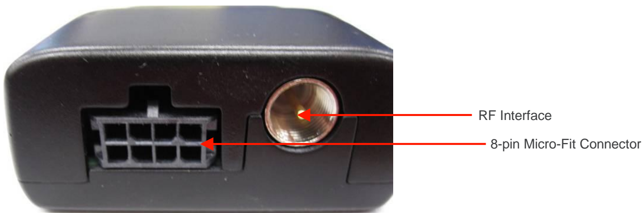
Figure 21. GL61x0 Back Interface
