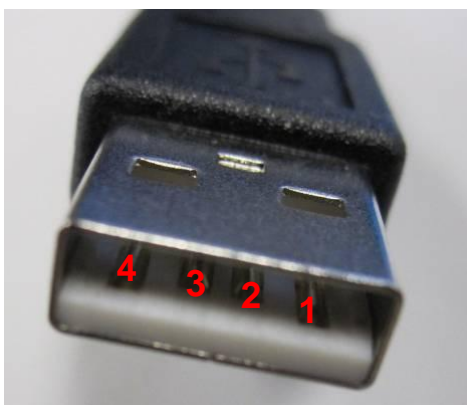
Figure 28. USB Signals on the USB Type A Connector
