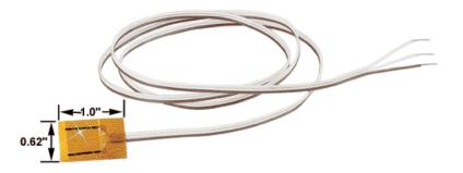
Models SRTD-1 and SRTD-2 are polyimide insulated surface mount RTD temperature sensors designed to provide a practical method for measuring surface temperatures. These sensors are small and flexible, and their low mass has minimal thermal effect on the material being measured. They are ideally suited for applications where the sensor can be mounted to the surface being measured using adhesives (OMEGABOND® 101 and 200 epoxies can be used) or other mechanical mounting methods.
