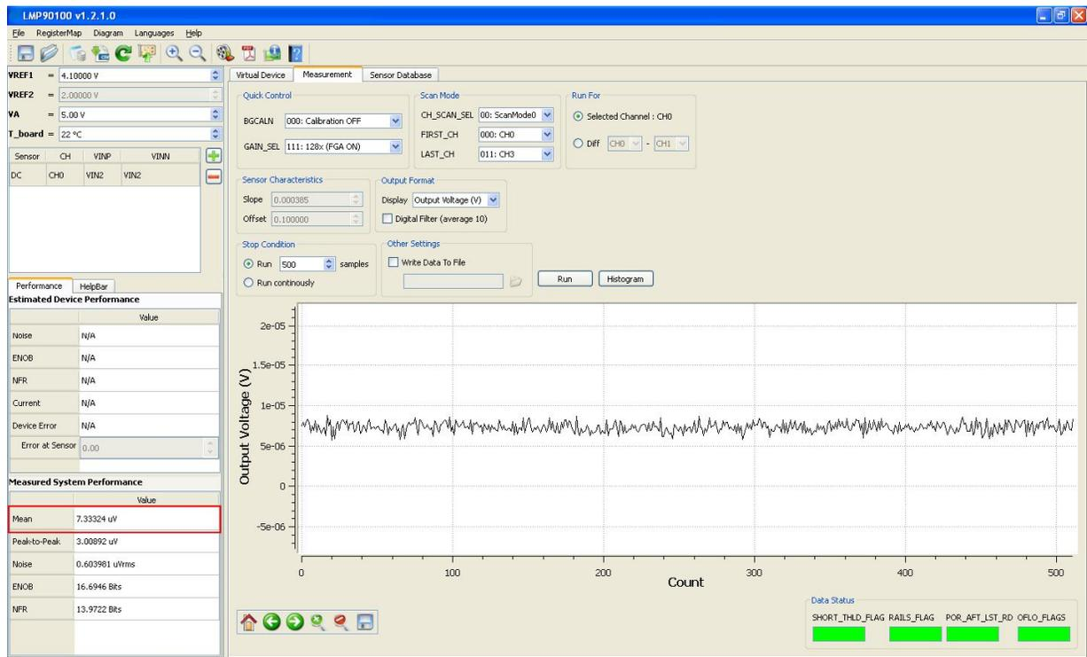
Figure 11 - Results for Shorted Input Test without Calibration
