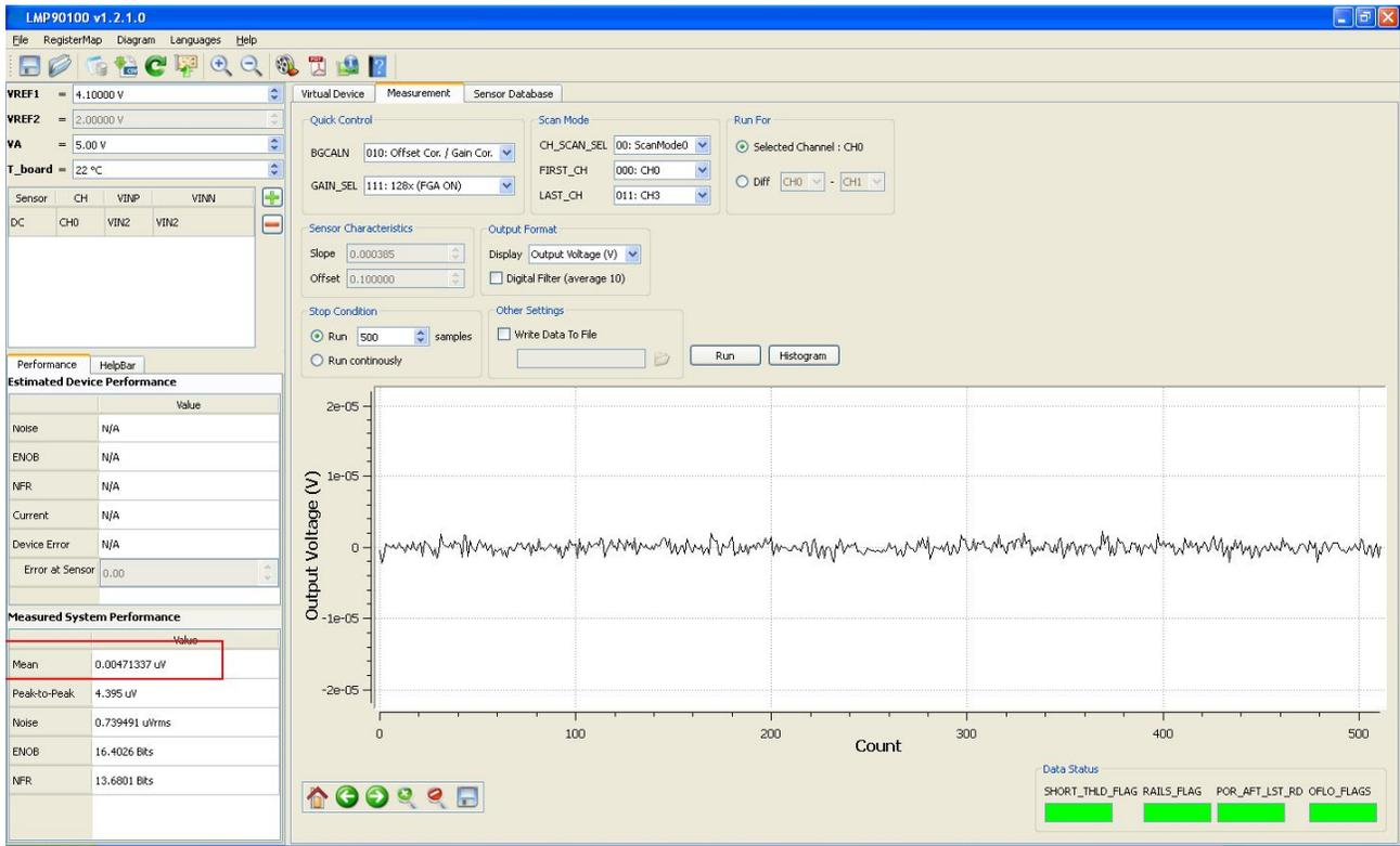
Figure 12 - Results for Shorted Input Test with Calibration
