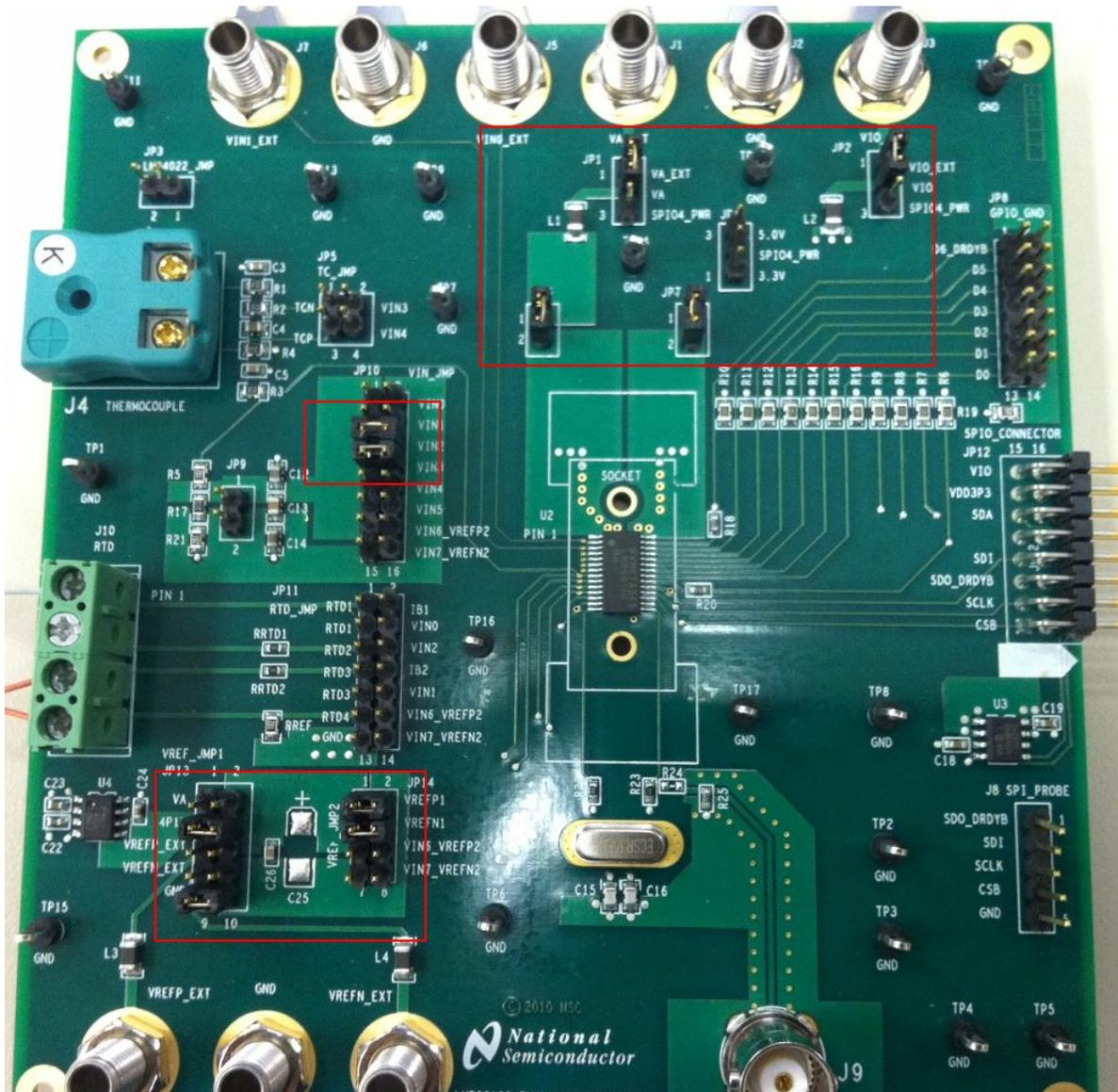
**Figure 3 – Jumper Settings (Default) for the DC Test**
