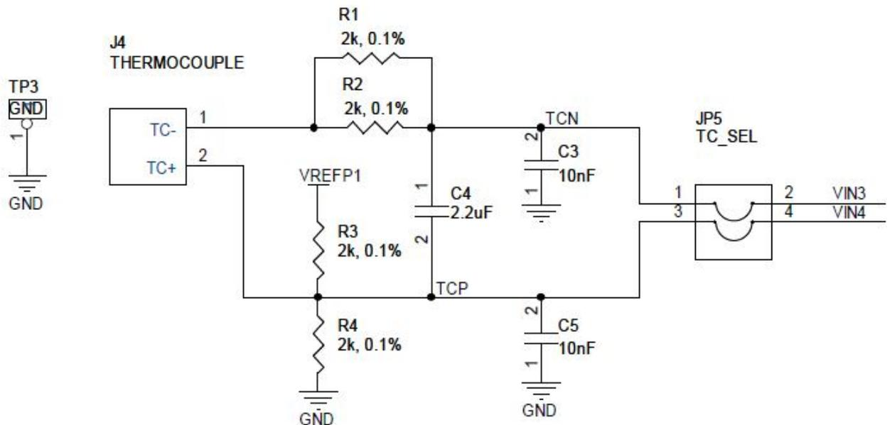
Figure 19 – Thermocouple and Temperature Sensor Schematic
