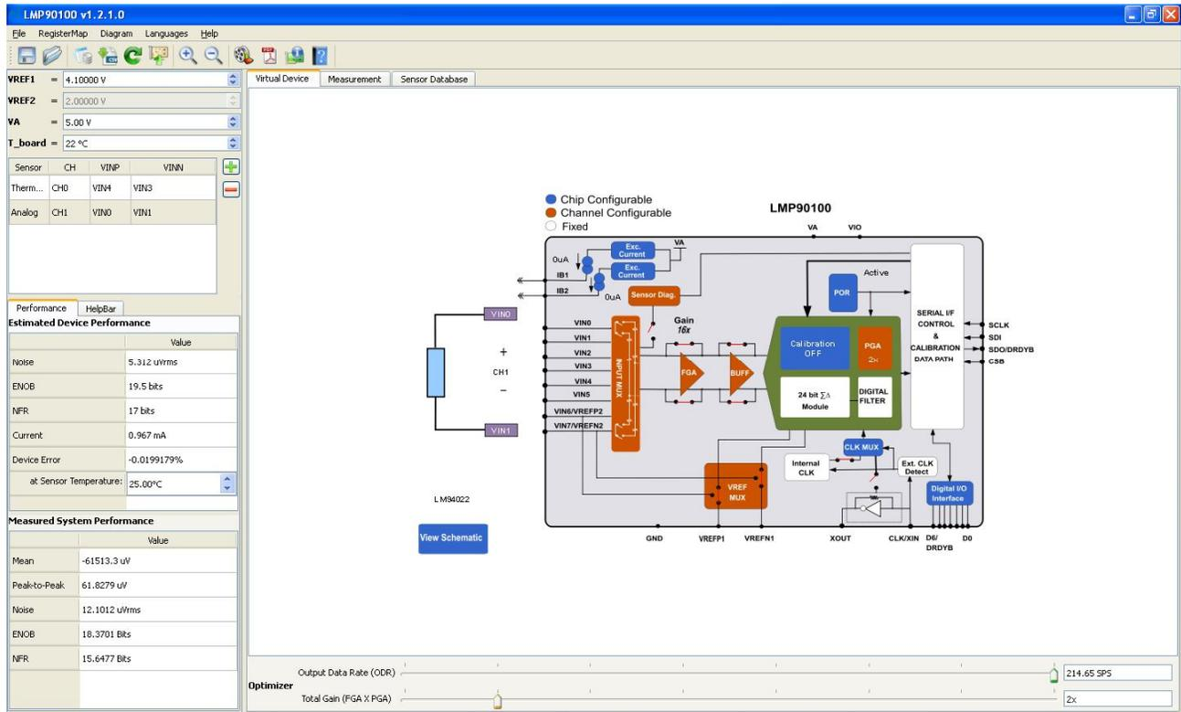
Figure 22 - Recommended LMP90100 Configuration for the LM94022
