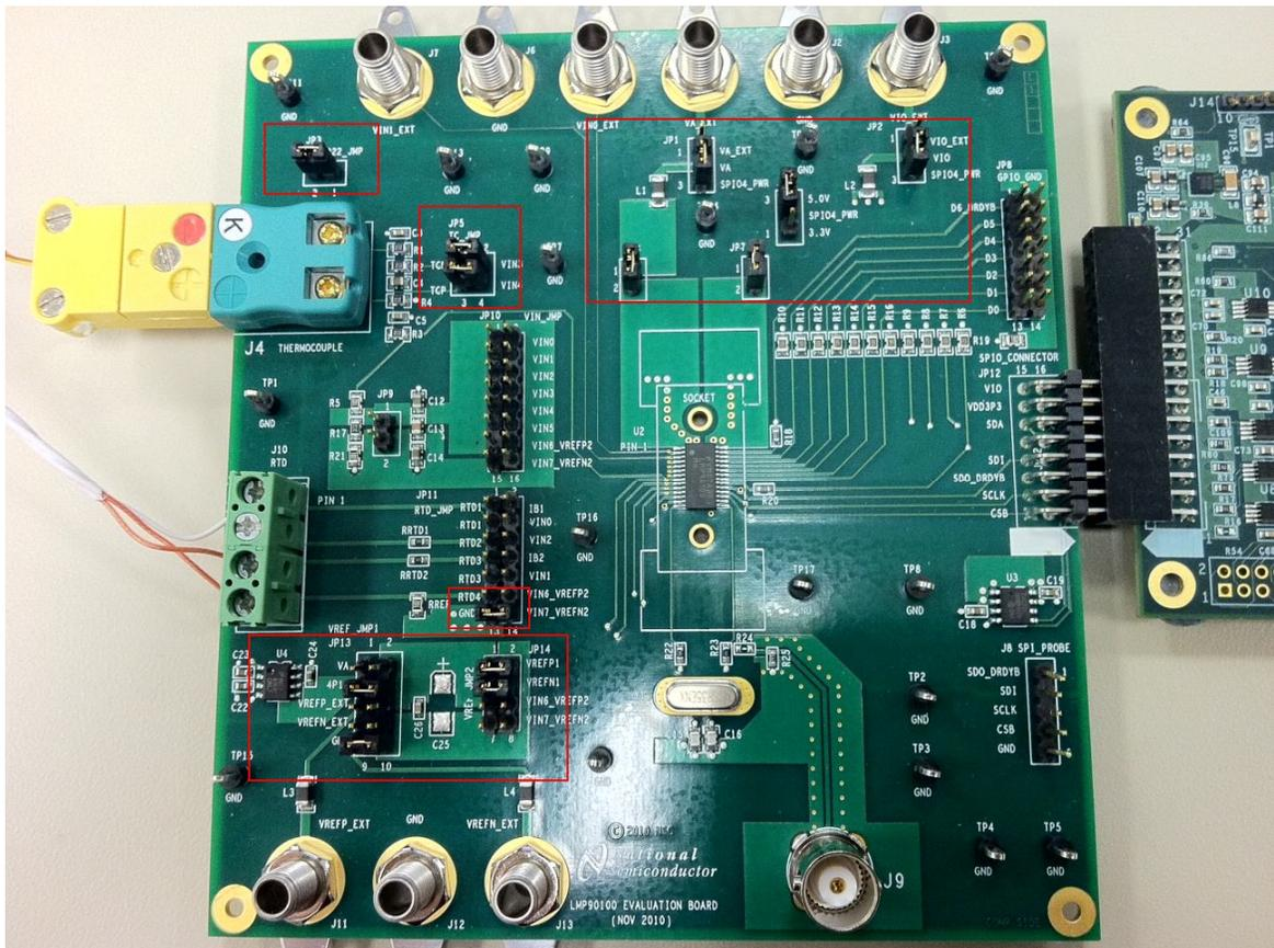
Figure 20 – Jumper Settings for the Thermocouple and LM94022 Example
