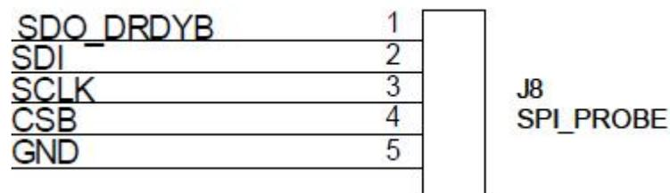
Figure 27 - LMP90100EB's J8 for SPI Signals
