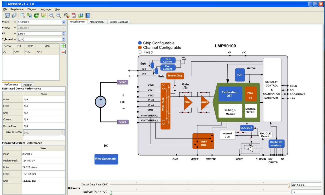
Figure 5 - Recommended LMP90100 Configuration for a DC Reading
