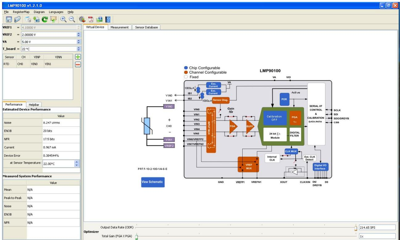
Figure 16 - Recommended LMP90100 Configuration for a PT-100 RTD Reading
