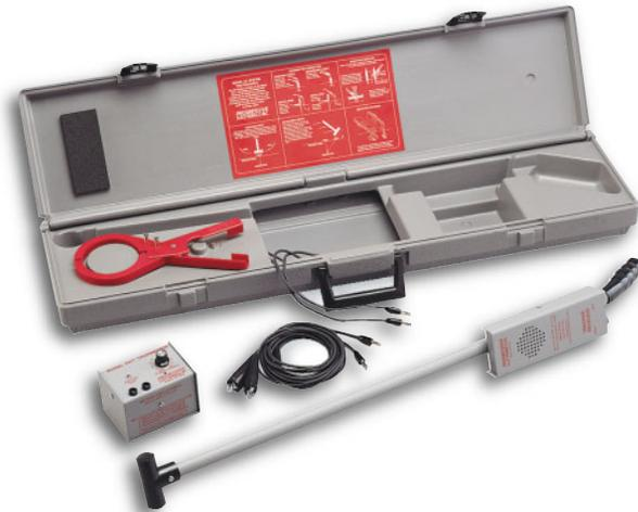
Traces the path and determines the depth of wires and metallic pipes on active or dead systems without having to deactivate the system.
