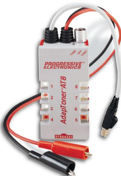
The AT Tone Generator makes it simple to test continuity, polarity, send tone and even supply talk battery to any configuration of pairs in 8-position modular jacks and plugs.
