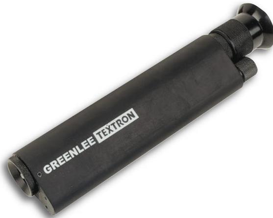
High-powered microscope is used to check a connector's endface for excess epoxy, core or cladding chips or other irregularities that degrade optical performance of the connector.
