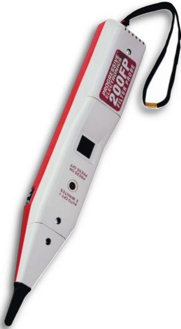
By selectively filtering out all 60Hz and 60Hz harmonics, the 200FP can be used with any tone generator for faster, more accurate, cable and wire identification.
