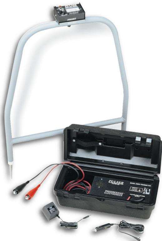
Identifies the exact location of even the smallest breaks in insulation by "pulsing" a high-voltage signal that radiates into the earth at the location of the faults. With the A-frame mounted receiver, a visual analog meter points the way to the source of the voltage.
