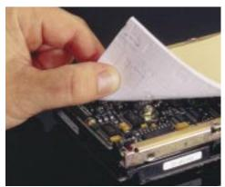
Gap Pad V0 is a thermally conductive material that acts as a thermal interface between a heat sink and an electronic device. The conformable nature of Gap Pad V0 allows the pad to fill in air gaps between PC boards and heat sinks or a metal chassis.
