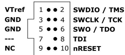
The following table lists the output of the 9-pin Cortex-M connector.
