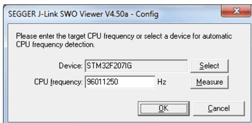
J-Link SWO Viewer automatically performs the necessary initialization to enable SWO output on the target.
