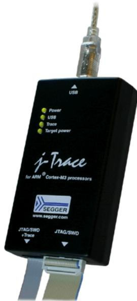
J-Trace for Cortex-M is a JTAG/SWD emulator designed for Cortex-M cores which include trace (ETM) support. J-Trace for Cortex-M can also be used as a regular J-Link and it also supports ARM7/9 cores. Please note that tracing on ARM7/9 targets is not supported by J-Trace for Cortex-M. In order to use ETM trace on ARM7/9 targets, a J-Trace is needed.
