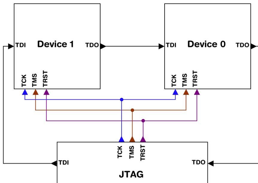
Currently, up to 8 devices in the scan chain are supported. One or more of these devices can be ARM cores; the other devices can be of any other type but need to comply with the JTAG standard.
