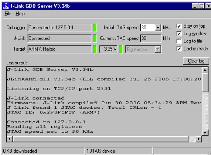
The GNU Project Debugger (GDB) is a freely available debugger, distributed under the terms of the GPL. It connects to an emulator via a TCP/IP connection. It can connect to every emulator for which a GDB Server software is available. The latest Unix version of the GDB is freely available from the GNU committee under:
