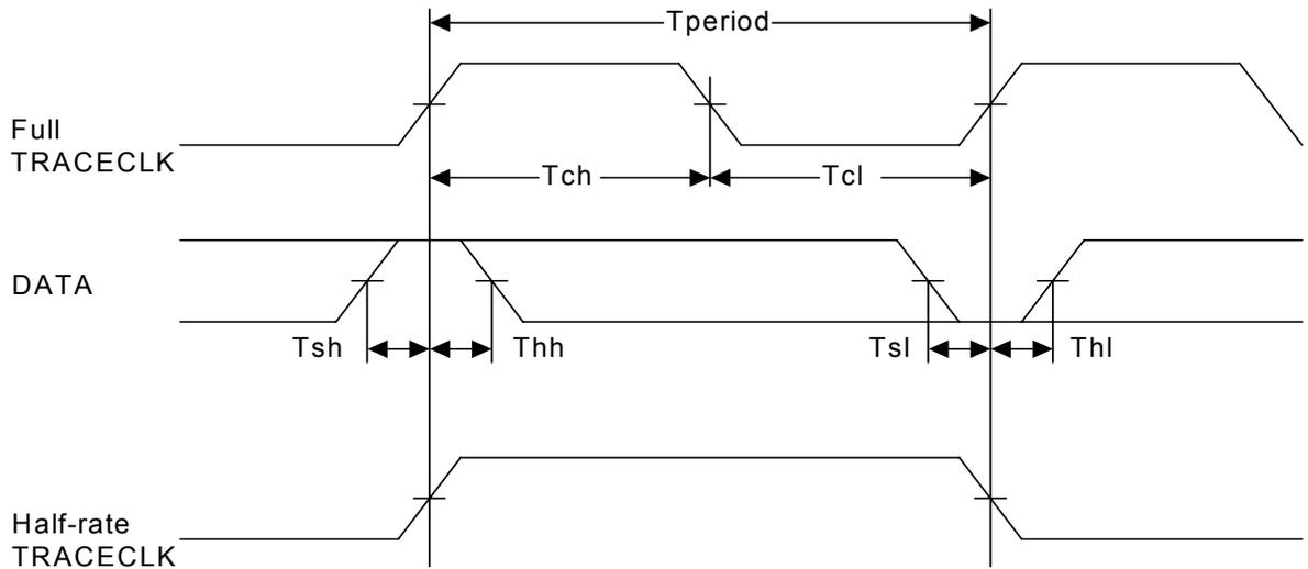
**Note:** J-Trace supports half-rate clocking mode. Data is output on each edge of the TRACECLK signal and TRACECLK (max)  $\leq$  100MHz. For half-rate clocking, the setup and hold times at the JTAG+Trace connector must be observed.
