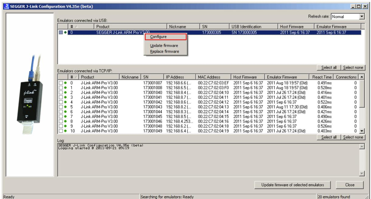
In order to configure a J-Link to use the new USB identification method (reporting the real serial number) simply select "Real SN" as USB identification method and click the OK button. The same dialog also allows configuration of the IP settings of the connected J-Link if it supports the Ethernet interface.
