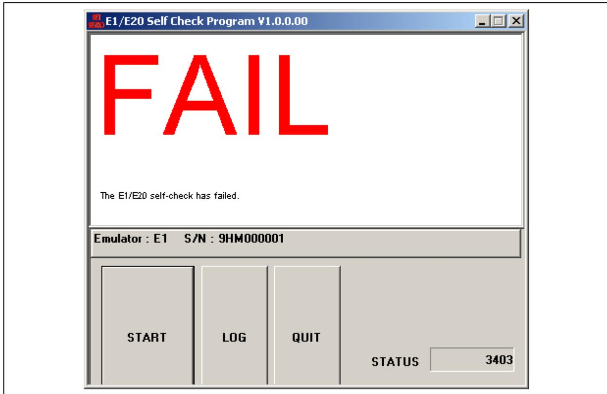
**Figure A.11 Display for an Error Found in Self-Checking**
