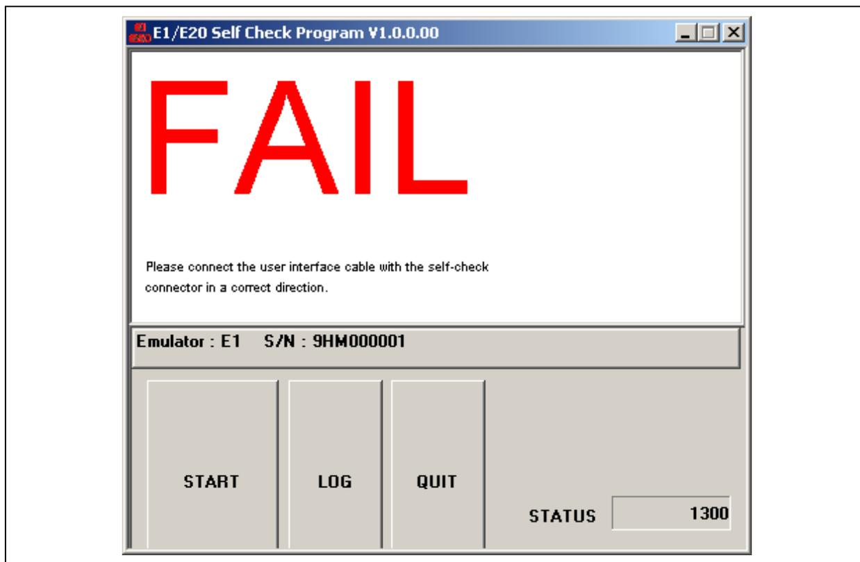
**Figure A.4 [FAIL] at the Start of Self-Checking
