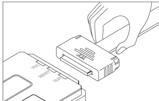
(1) A connector to the user-system interface cable must be installed on the user system. Table 2.1 shows the recommended connector for the emulator.
