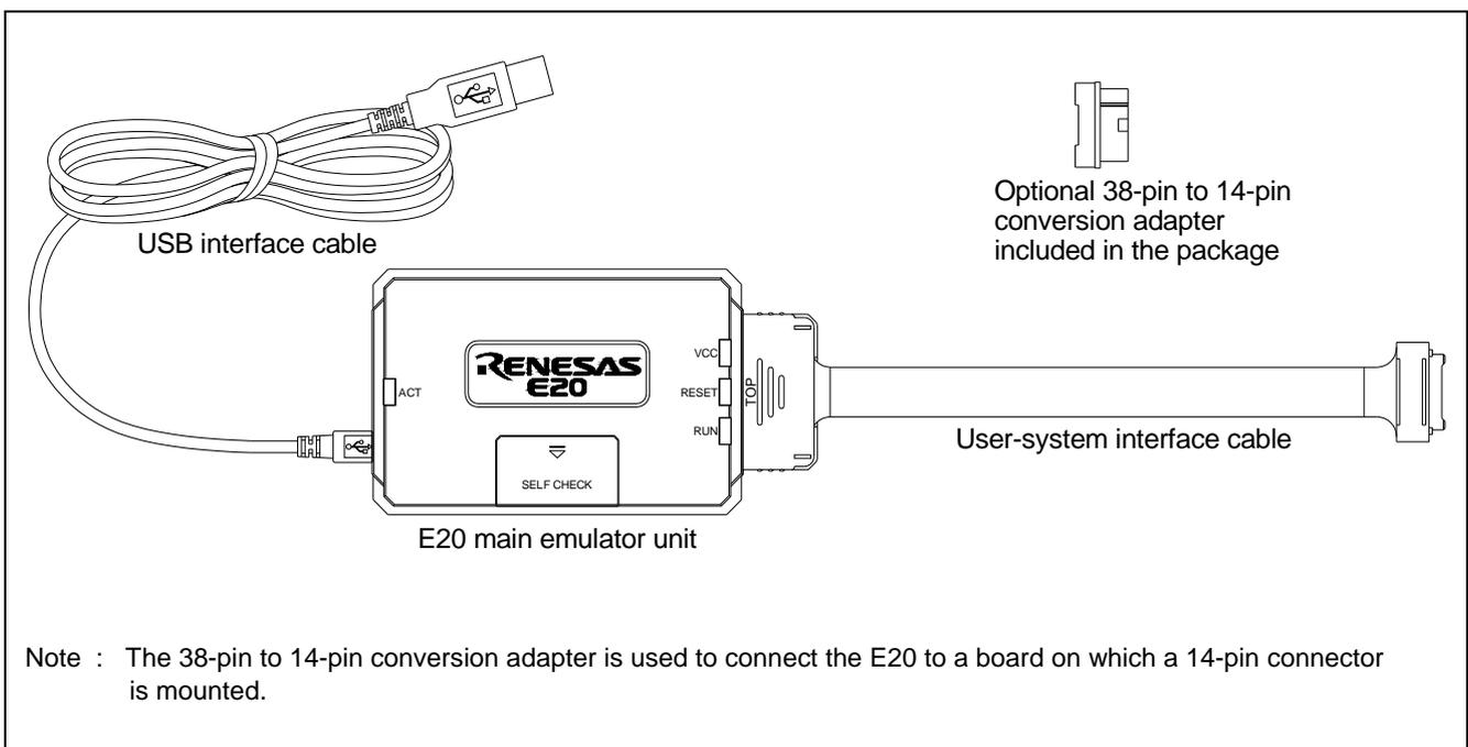
Note : The 38-pin to 14-pin conversion adapter is used to connect the E20 to a board on which a 14-pin connector is mounted.
