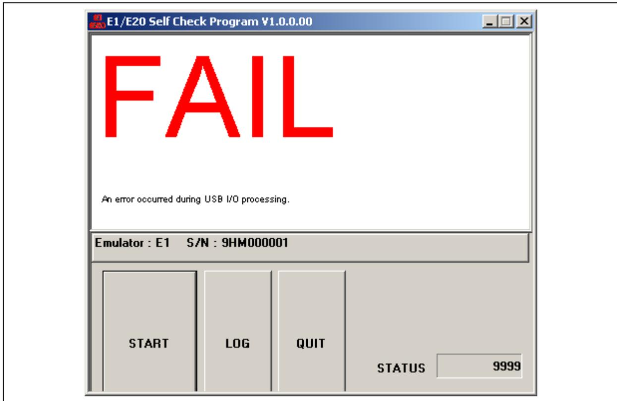
Figure A.6 [FAIL] on Error with USB I/O Processing
