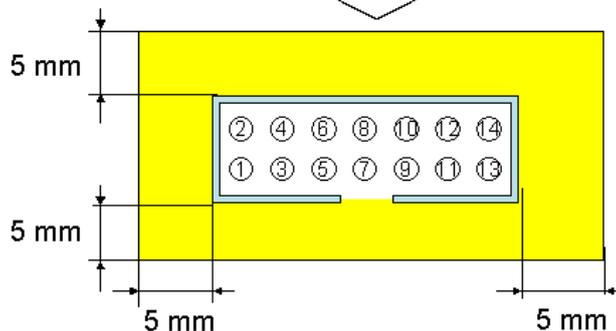
Area with limit on mounted components (heights must be no greater than 10 mm)
