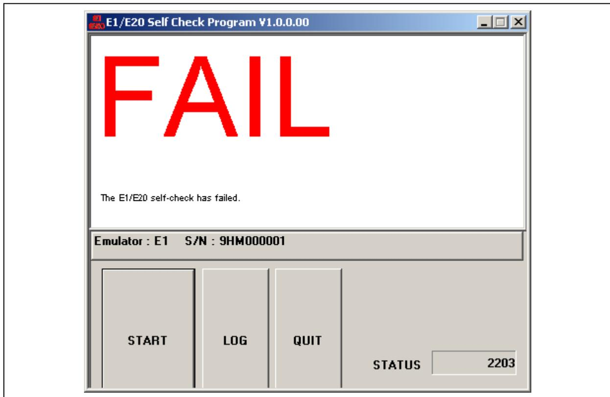
Figure A.5 [FAIL] at the Start of Self-Checking (with the Cable Connected to the User System)
