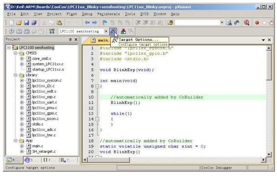
2) "Debug -> Use", open the configuration dialog and selects "CooCox Debugger".
