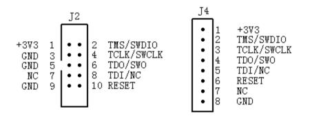
J2 is compatible with the standard ARM 10 PIN SW/JTAG Interface. So if you have the 10pin(2mm) to 20pin(2.54mm) connector, you can use it to connect J2 to ARM 20-PIN Interface directly.
