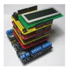
The Cookie, like the Arduino, features a common footprint for expansion headers that are intended to allow connectivity with a large number of expansion daughter cards called "shields". The shields have been developed by both the original Arduino
