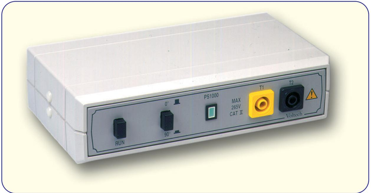
The Voltech PS1000 solid-state switch controls the turn-on of an AC supply to allow accurate measurement of the inrush current into an AC load. It is designed for use with Voltech power analyzers such as the PM100, PM300 or PM3000A.
