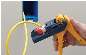
4. Ensure jack is completely and securely inserted in jack holder bed with IDC slots facing the blades.
