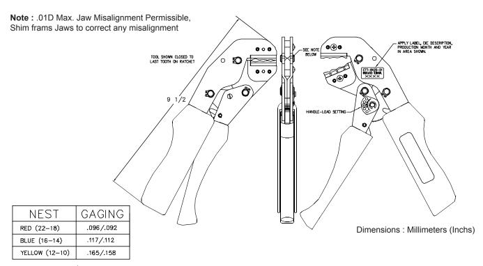
GAGING USING CO/NO CO PNS WITH TOOL CLOSED TO LAST TOOTH OF RATCHET
