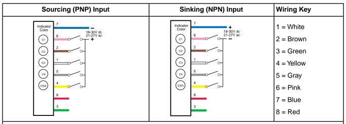
Pin 4 could activate the corresponding color or the audible function, depending on model. Pins 3 and 8 are not used.
