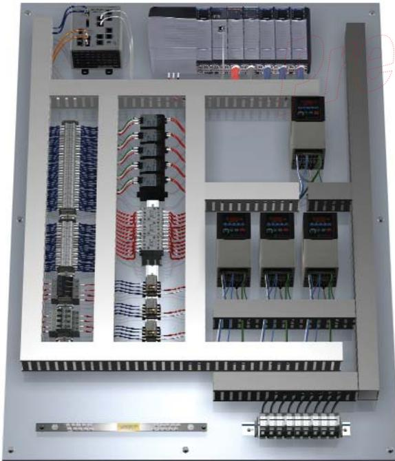
Conventional panel layout relies primarily on air spacing between pathways and components to mitigate noise. Duct color is used to indicate noisy (gray) and clean (white) pathways.
