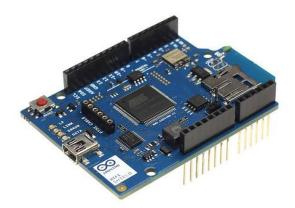
The Arduino WiFi Shield connects your Arduino to the internet wirelessly. Connect it to your wireless network by following a few simple instructions to start controlling your world through the internet. As always with Arduino, every element of the platform – hardware, software and documentation – is freely available and open-source. This means you can learn exactly how it's made and use its design as the starting point for your own circuits.
