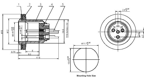
The pin plating gold, thickness 0.05µm (SOLDER).
