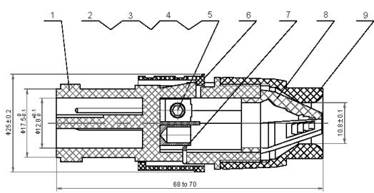
The pin plating nickel, thickness  $1\mu m$  (SOLDER+SCREW).
