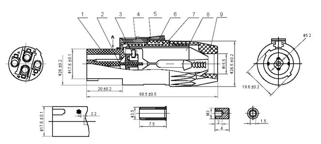
Pin with copper plating  $10\mu m$  first, and then silver plating  $4\mu m$  (SOLDER+SCREW).
