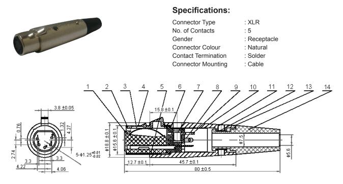
The female pin plating silver, thickness 0.5µm (SOLDER).
