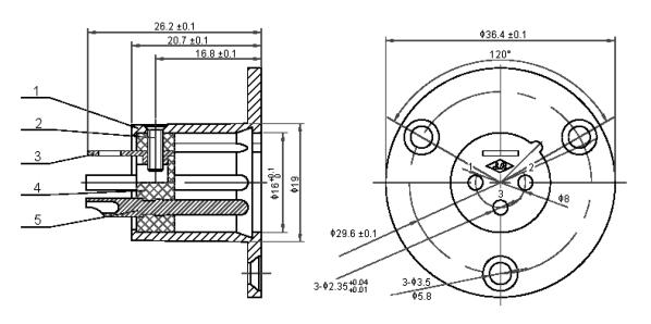
The pin plating silver, thickness 0.5µm (SOLDER).
