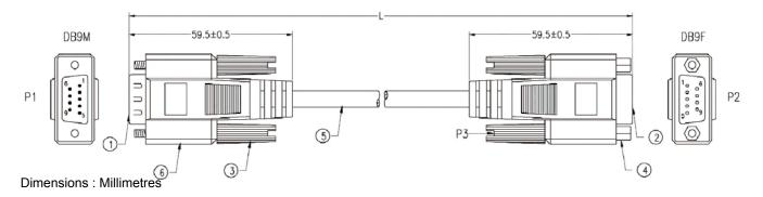
P1 P2 1 1 2 -2 3 — - 3 - 4 4 — 5 -- 5 - 6 6 -7 -\_\_\_\_\_ 7 8 \_\_\_\_\_ 8 - 9 9 -SHIELD \_\_\_\_\_\_ SHIELD
