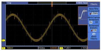
Output of DAC Signal – Notice how FilterVu<sup>TM</sup> clearly shows the noise-free steps of the DAC in the foreground trace (yellow) which has removed all frequencies above 5.5 kHz. FilterVu also captures and displays high-frequency glitches up to the full bandwidth of the oscilloscope in the background trace (orange).
