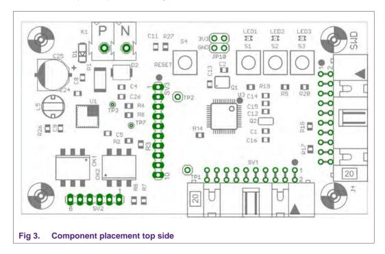
The upper left part of the board contains the KNX TP1 header K1 to connect the KNX bus. Below the KNX connector, the board contains the physical transceiver part of the design. On the left bottom side the isolated UART interface is available on header SV2.
