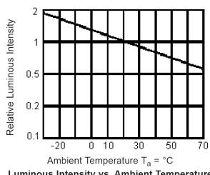
**Luminous Intensity vs. Ambient Temperature**
