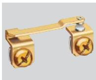
One piece rivetless copper alloy spring contact arm and terminal plate assures proper contact alignment reducing heat rise. Large silver cadmium oxide contacts reduce contact erosion and prevent welding, providing long life.
