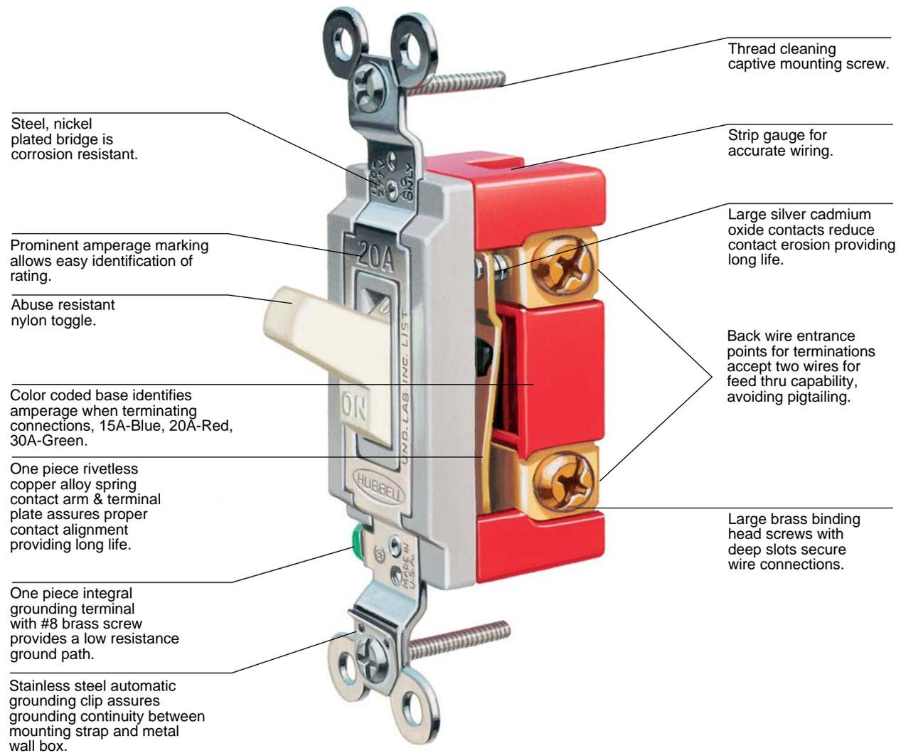
Steel, nickel plated bridge is corrosion resistant.
