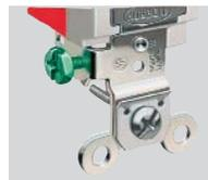
One piece integral grounding terminal with #8 brass screw allows compliance to NEC®. Stainless steel automatic grounding clip assures grounding continuity between mounting strap and metal wall box. Steel nickel plated mounting strap provides a corrosion resistant finish.
