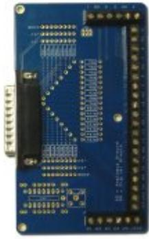
With as many as seven bipolar voltage ranges, the ADC-20 and ADC-24 are also flexible enough to be used with a wide range of sensors and signal types. Whilst the optional terminal board provides screw terminals to allow you to quickly connect and disconnect different sensors.
