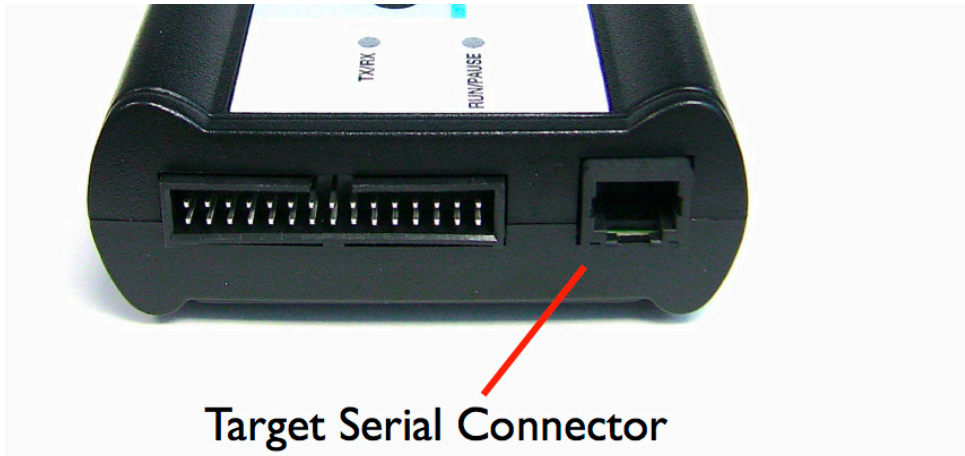
Figure 5.5 CW TAP Probe — Target Serial Connector
