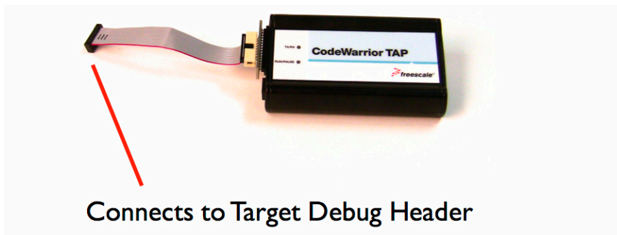
Figure 3.2 CW TAP Probe — Connecting to the Target
