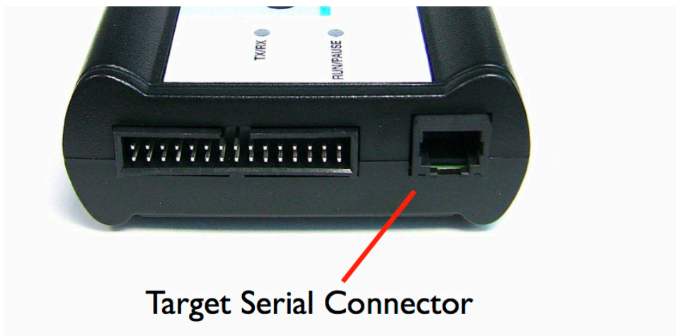
Figure 3.3 CW TAP Probe — Target Serial Connector
