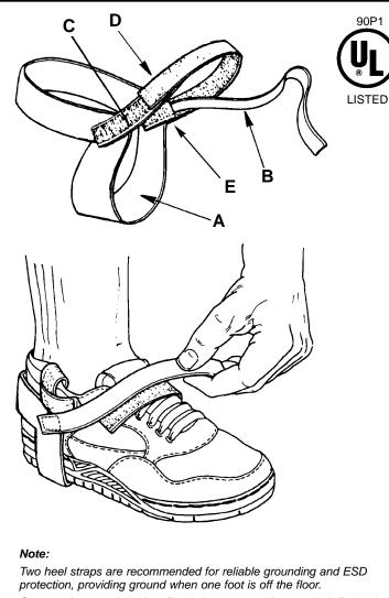
Operator is grounded when foot is in contact with grounded dissipative or conductive flooring.
