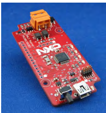
Fig 1. DALI Master assembled PCB
