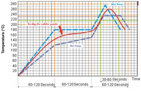
Infrared Soldering Profile
