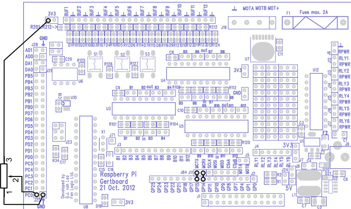
Figure 33: Wiring diagram for the sketch AnalogReadSerial.
