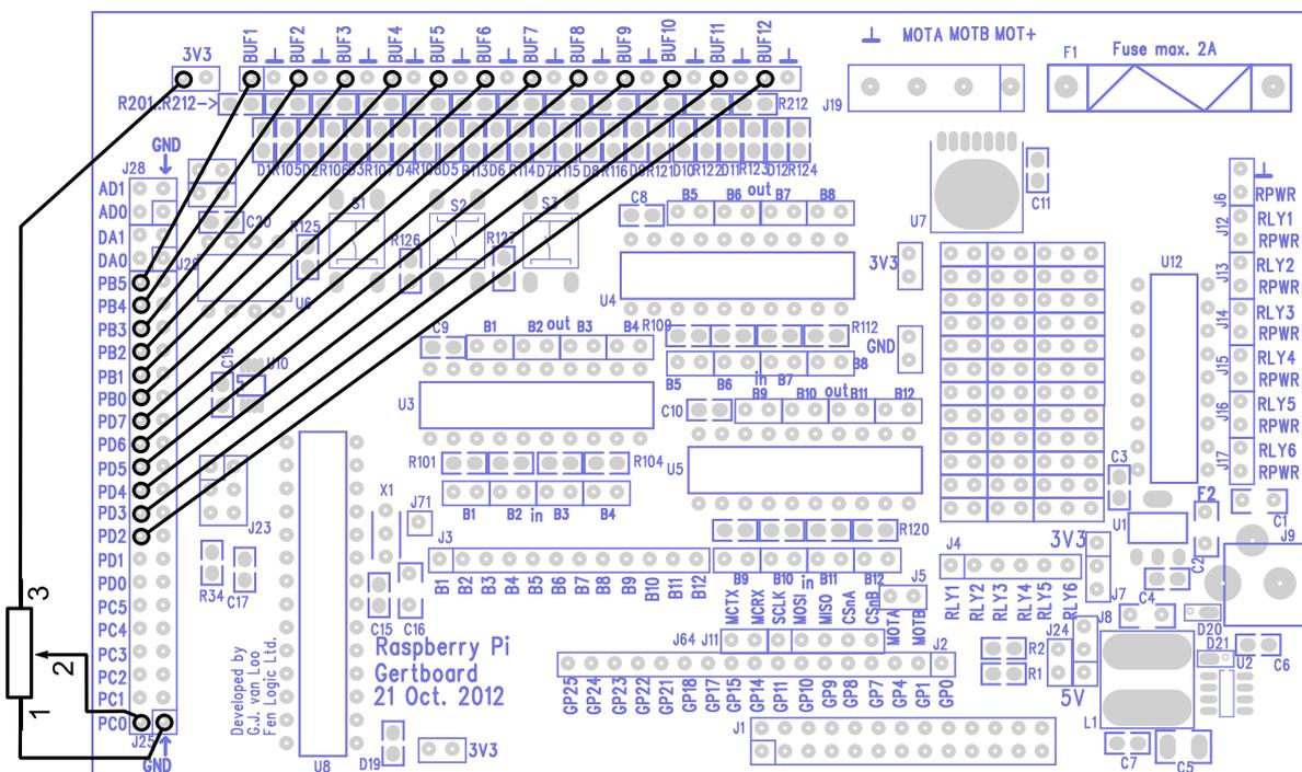
Figure 34: Wiring diagram for the LEDmeter sketch
