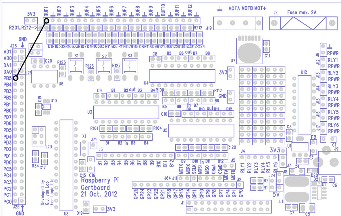
Figure 28: Wiring diagram for the sketch Blink.
