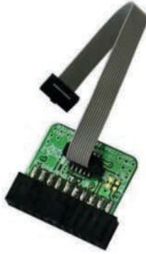
JTAG 20 PIN 0.1" TO 10 PIN 0.05" ADAPTER
