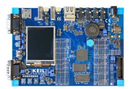
The Keil MCB1800 Evaluation Boards enable you to create and test working programs based on the NXP LPC1850 family of ARM Cortex $^{\text{TM}}$ -M3 processor-based devices.
